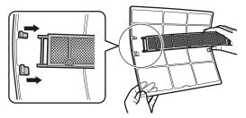
2 Remove the dust from the filter with a vacuum cleaner.
