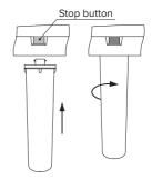
Figure 13. Installation of the membrane cartridge service plug
