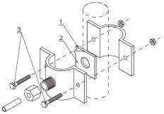
It is best install the drain saddle on the sink drain before the siphon trap or bend (the drain saddle on most drain pipes is of  $\sim$ 40 mm diameter).
