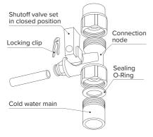
Figure 5. Connection node installation scheme
